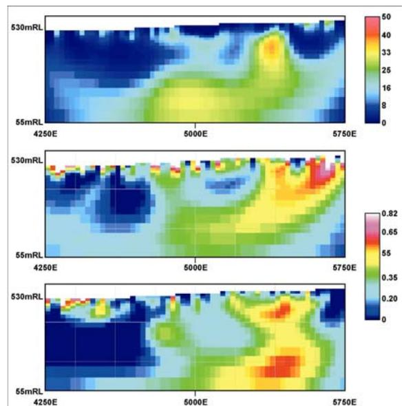
**Figure 4. Chargeability model sections for 2D2D (top), 2D3D (centre) and 3D3D (bottom) inversions – Line 4850N. Note that the 2D2D has not detected the moderate east dipping structure in the centre of the section and the poor resolution of a parallel structure (eastern end of sections) in both 2D2D and 2D3D.**
